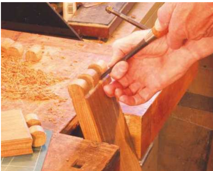
▲ Pic.13 Final cleaning of the hollows
